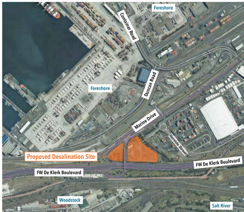
Water, water, everywhere, and soon it'll be safe to drink! An aerial picture showing the proposed location (highlighted in orange) of the permanent desalination plant in Paarden Eiland. The plant will have a water production capacity of 50-70 million l/day.
